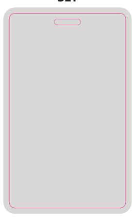
Overall Dimensions – 2.5" X 4.188" Slot Punch – .5625" X .125" Gray Indicates Bleed Area – .125" All Around Die – ADC3-241
